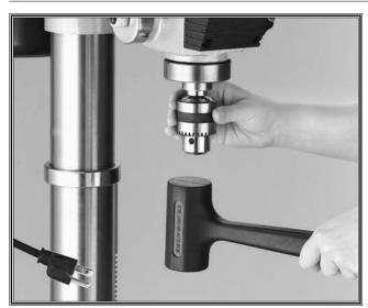
Figure 20. Seating arbor into spindle.
